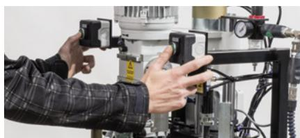
6 spindle drilling head for drilling holes for hinges, mounting plates and fixtures and fittings
