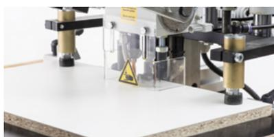
Pneumatic two-hand control for fast, safe working
