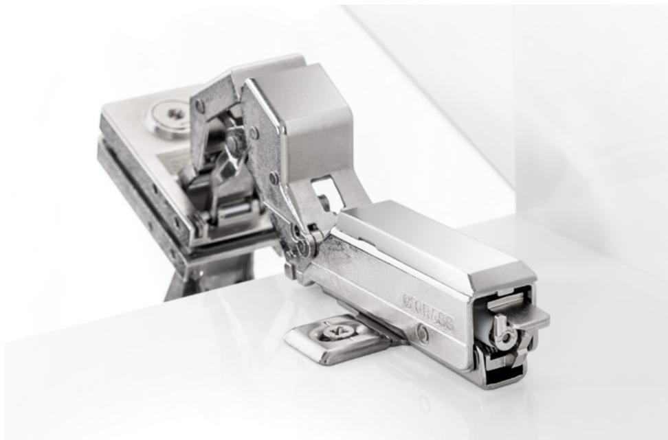
Tiomos Mirro is secured on the glass side of the door with an eccentric cam on a Zamak adapter. It is not necessary to drill a hole in the glass. This fastening method ensures firm attachment and has a light, floating look.
